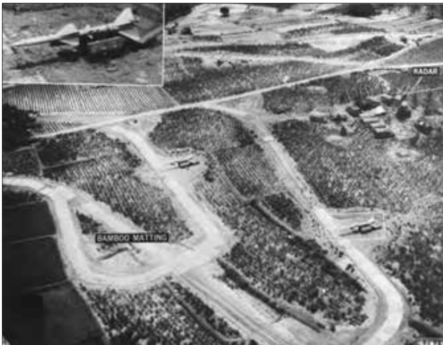
A North Vietnamese SA-2 surface-to-air missile site. The SA-2 had a maximum range of about 31 miles, a maximum operating altitude of 80,000 feet, and speed of Mach 3.5. It usually carried a high explosive warhead of 287 pounds. During the course of the war, the Navy developed various methods for defeating SAMs, including defensive maneuvering, electronic countermeasures, and hunter-killer teams armed with antiradiation missiles.
